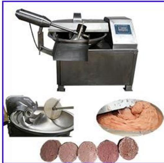
**Bowl Cutter** uses high rotating chopping knife to cut the meat granular which is from meat grinder, while the chopper pan is rotational of a low velocity.
