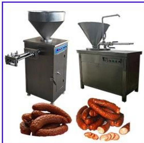
This Sausage stuffing machine is suitable for sausage filling with natural sausage casings, collagen casing and Smoked sausage casing. Continuously and automatically quantitative filling and twist is the most advantage.
