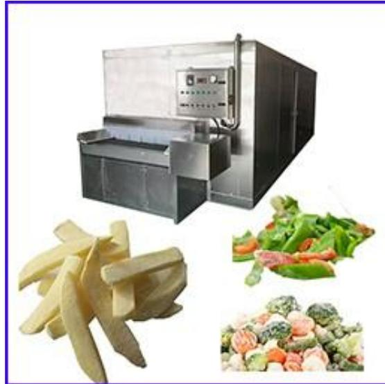
Quick freezing is rapid freeze of food by exposure to a blast of air at a very low temperature. Unlike slow freezing, very small crystals of ice are formed which do not rupture the cells of the food and so the structure is relatively undamaged.
