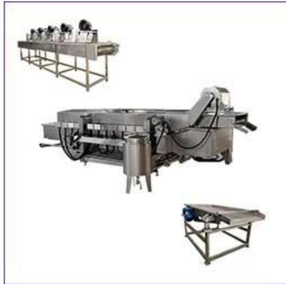
The high quality demands equal color of the stick and prevention of after cooking darkening. Before the chips or fries are fried, it should be properly dried. **Potato chips air drying machine** conveyer chips or fries with air blowing while chips turnover, the surface water will be removed completely and quickly, the dryer has to remove a certain amount of the water from the product to improve crispiness of the stick and shorter frying times.
