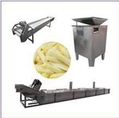
After potato peeling process, hand picking will be done on a sorting table to select the defective potatoes. And then up-to-standard potatoes will be collected in receiving hopper which has a buffer for at least 10 minutes to cope with fluctuations in the feed.
