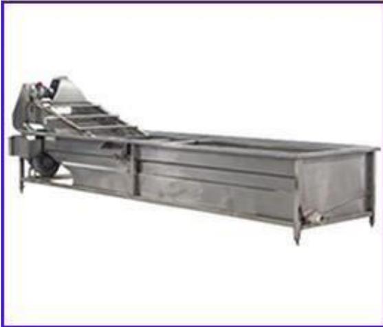
The slices fall into a cold-water air bubble washer that removes the starch released when the potatoes are cut. Some manufacturers, who market their chips as natural, do not wash the starch off the potatoes.
