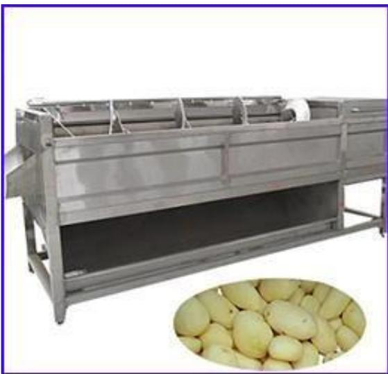
Both batch potato chips production line and potato chips industry manufactures, potato peeling must be the necessary step. Potato peeler machine ensures optimum peeling. The less peel is removed, the higher the yield of your process.
