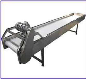
After potato peeling process, hand picking will be done on a sorting table to select the defective potatoes. And then up-to-standard potatoes will be conveyed to next process, chips or fries cutting and slicing.
