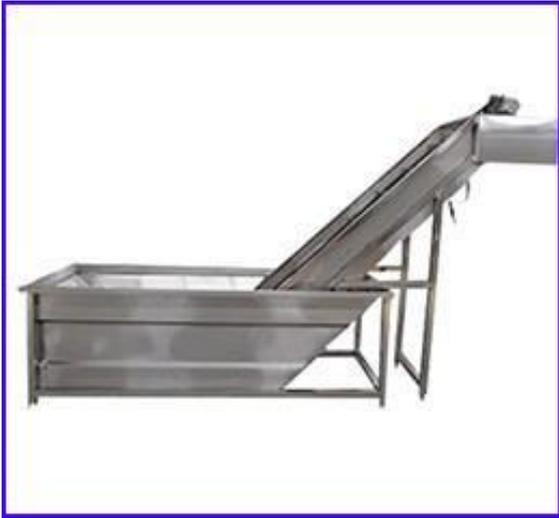
The potatoes move along a potato elevator to potato peeling machine, there are a sediment design in the feeding water sink. The sediment on potatoes is precipitated and discharged through the sewage exit while conveyers.
