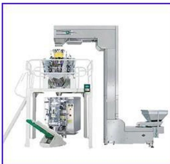
The chips are conveyed to a chips automatic packaging machine with a scale. As the pre-set weight of chips is measured, a metal detector checks the chips once more for any foreign matter such as metal pieces that could have come with the potatoes or been picked up in the frying process.
