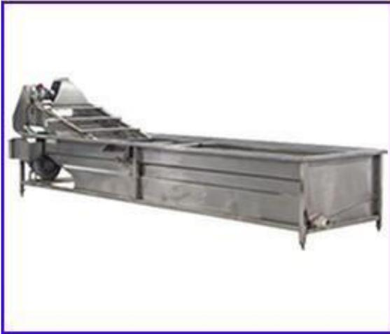
Potato chips and fries will have some extra temperature after blanching process, sometimes adhesion problem of chips and fries will happens. Cooling machine which uses the up and down air bubble will completely broke up the chips and fries while the temperature will drop immediately, at the same time, excessive blanching for chips and fries will be avoid.
