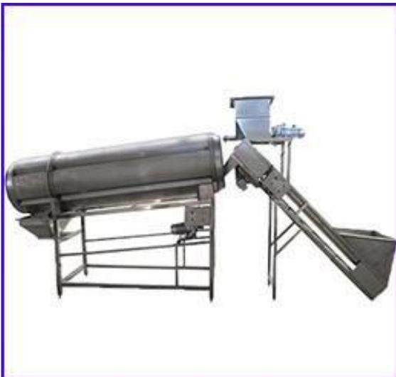
Potato chips that are to be flavoured pass through a drum potato chips fries flavoring machine which is filled with the desired powdered seasonings. to meet different customer demand for potato chips, hot chips, finger chips, fries, frites, potato wedges.
