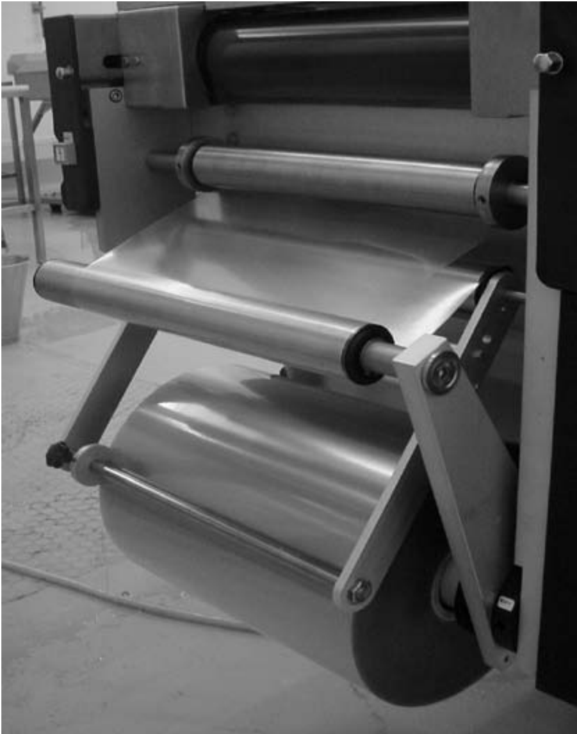
Figure 10.8 Lower web unwind and infeed section on the Multivac R230.
